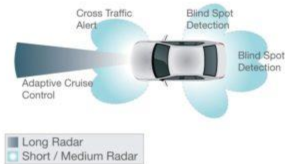
Figure 2: Radar in a car can be short- or long-range. This illustration shows some of the applications for the long-range (dark blue) and short-range (light blue) radars.
